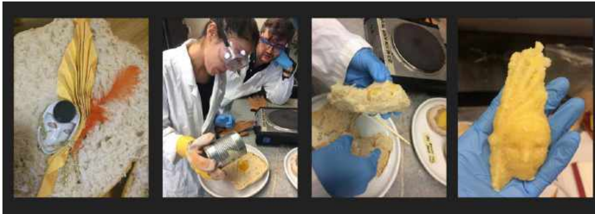
Figure 2: L to R, A model is pushed into moist bread pith; molten sulfur or wax is poured into the hollow; once hardened, bread is broken away from the cast wax or sulfur; the impression is revealed.
